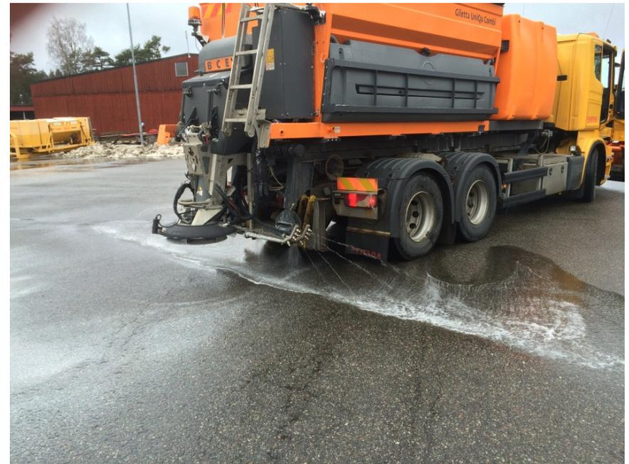
**A new satellite assisted GPS controller that controls, material dispensing, liquids, the front plow and the wing plow. The operator just drive!**
