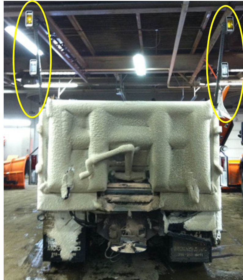
Rear warning lights mounted on the telespars, showing snow accumulation (NDDOT).
