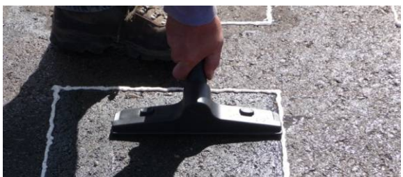
FIGURE 35 Sampling boxes shown (a) after addition of de-ionized water and (b) during the agitation step.
