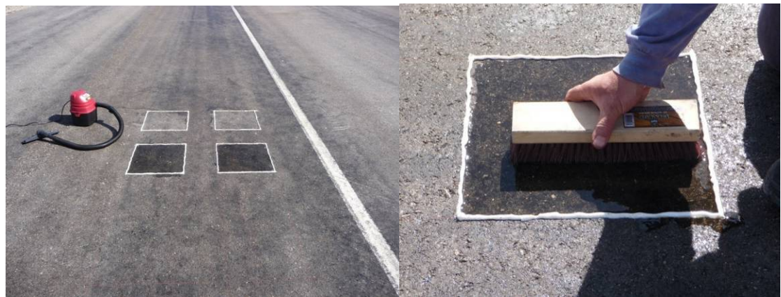
FIGURE 35 Sampling boxes shown (a) after addition of de-ionized water and (b) during the agitation step.
