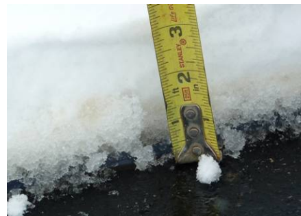
FIGURE 52 Photo showing the upward migration of deicer up to 2 inches of snow cover.
